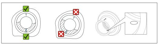
$\blacksquare 19$  Weld-in adapter with leakage hole
