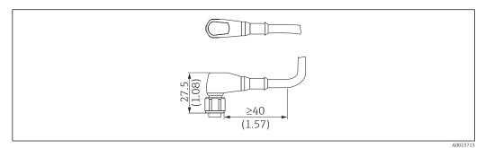
■ 44 Plug-in jack M12 IP69. Unit of measurement mm (in)
