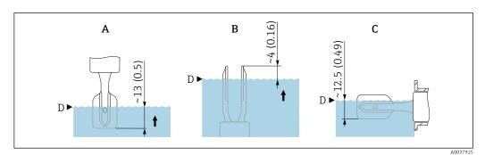
₽8 Typical switch points. Unit of measurement mm (in)
