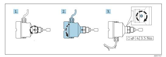
$\blacksquare 17$  Housing with external locking screw and drip loop
