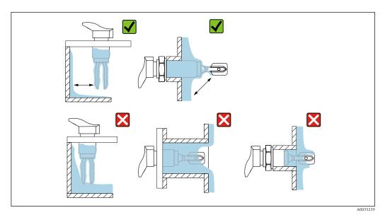
Installation examples for a highly viscous process medium
