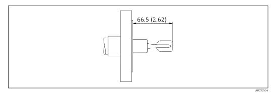
■ 39 Example with flange. Unit of measurement mm (in)
