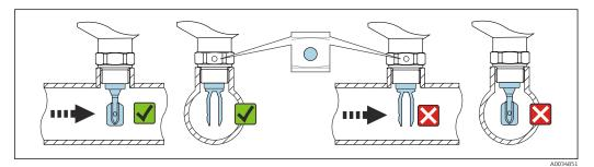
*Installation in pipes (take fork position and marking into consideration)*
