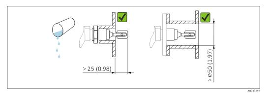
■ 11 Installation example for low-viscosity liquids. Unit of measurement mm (in)
