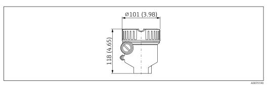
■ 25 Single compartment; aluminum, coated; suitable for Ex d/XP area
