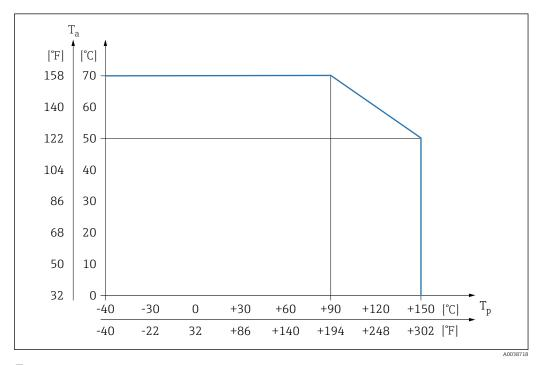
$\blacksquare$  20 At process temperature and FEL44  $T_p > 90$  °C max. load current 4 A
