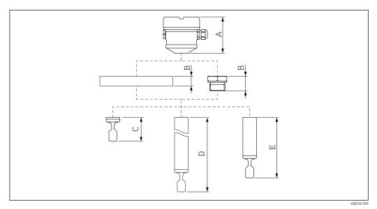
$\blacksquare$  22 Components to determine the device height
