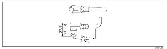
🛮 45 Plug-in jack M12 IP67. Unit of measurement mm (in)
