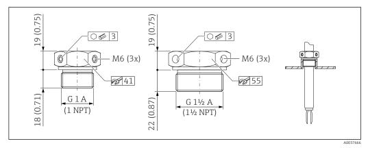
$\blacksquare$  46 Sliding sleeves for unpressurized operation  $p_e = 0$  bar (0 psi). Unit of measurement mm (in)
